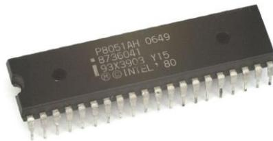
Gambar 2.6 Mikrokontroler Intel 8051 (Khadse, Gawai and Faruk, 2014)
