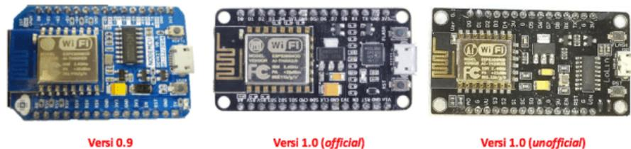
Gambar 2.10 NodeMCU ESP8255
